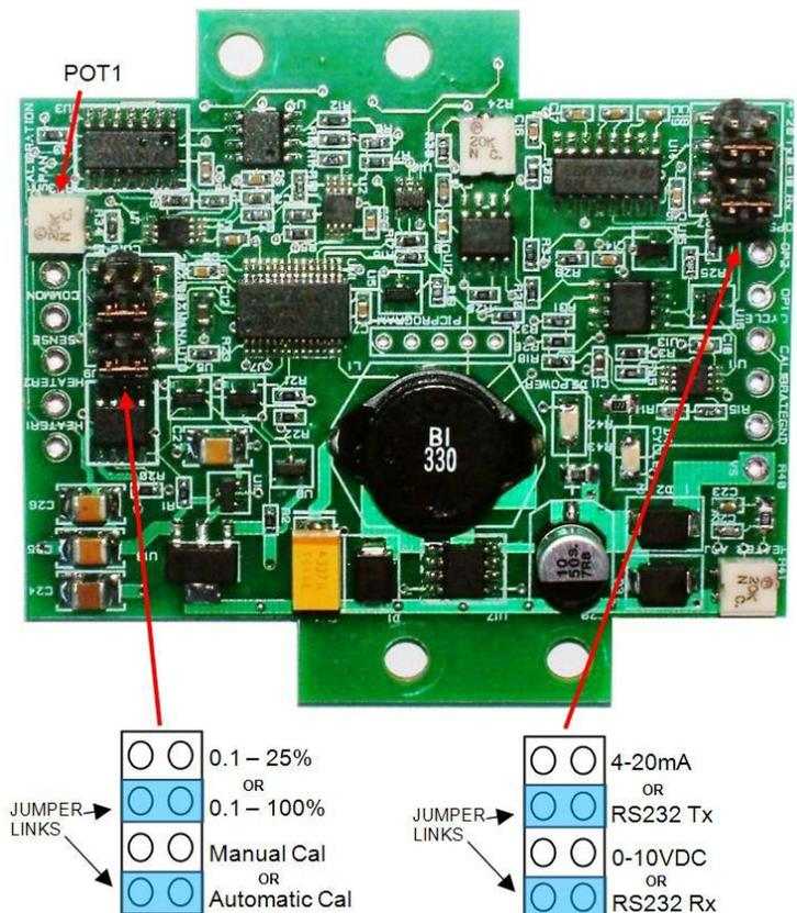
NOTE: Each Jumper Link must be placed in one of the two positions. When selecting the output, you must choose either 4-20mA and 0-10V<sub>DC</sub> or RS232 Tx and Rx. Ensure the Jumper Links are always inserted horizontally between 2 adjacent pins.
